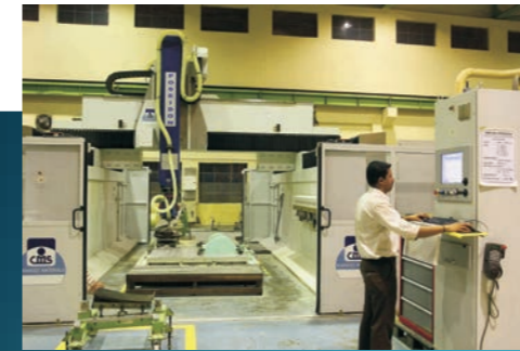
High precision 5 axis NC machine
